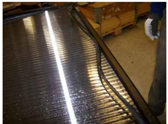
23. The rubber strip is then put in around the panel. Be aware that the rubber strip is "too long". This makes it possible to adjust itself when it's hot, cold etc.
