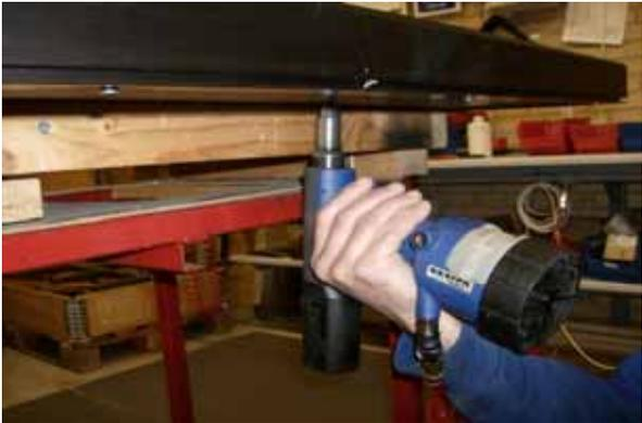
16. Pop rivets are put in from behind on the back plate.
