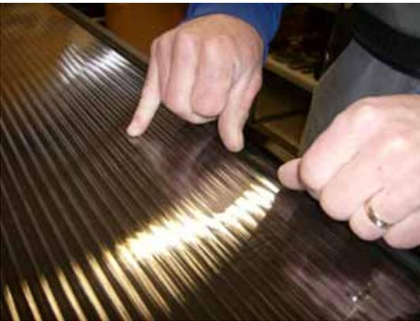
3. Loosen the rubber strip on the sides between the cover layer and the aluminum frame on the front.
