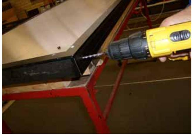
2. Drill out the pop rivets. Dimension of the bit - from 4 to 4.2 mm.
