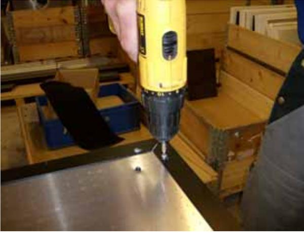
1. On the back side of the panel - unscrew the screws on the end gable opposite to the fan.
